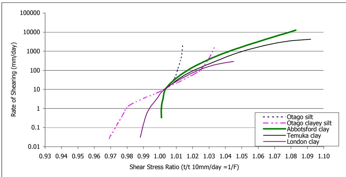
Figure 3a Residual Strength Dependence on Shearing Rate
