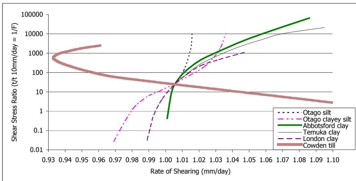
Figure 3b Residual Strength Dependence on Shearing Rate
