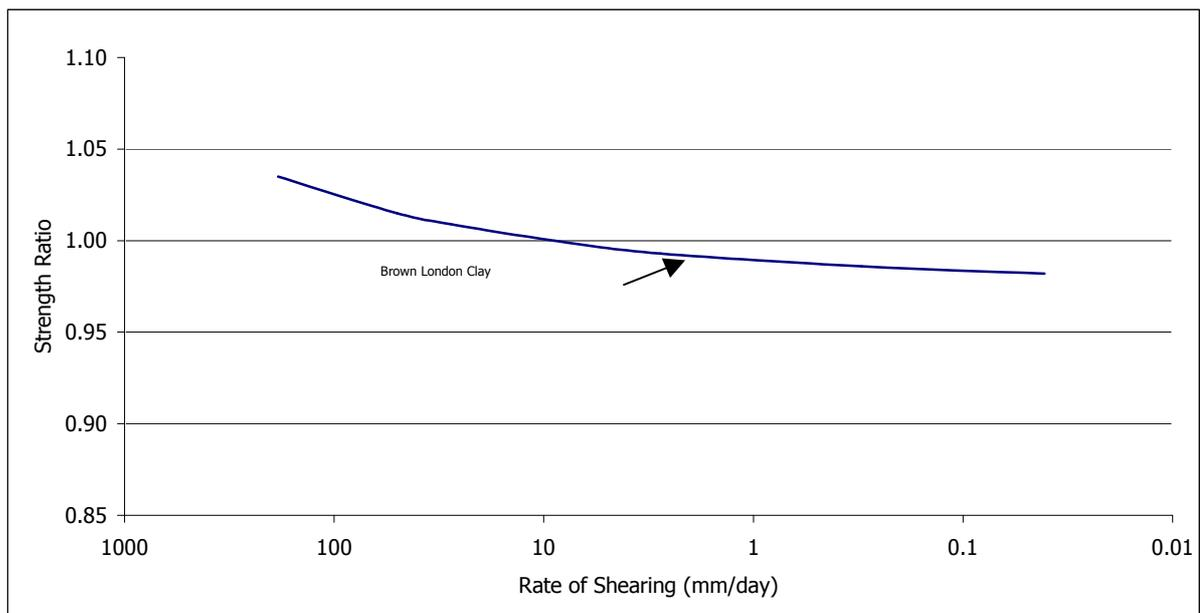
Figure 2a Rate Dependence of Residual Strength
