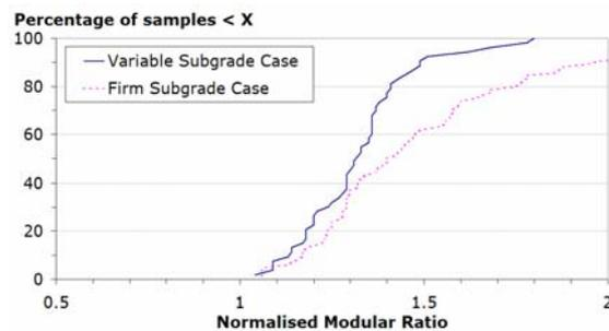
Figure 4. Cumulative Normalised Modular Ratio Distributions for New Trafficked Pavements.
