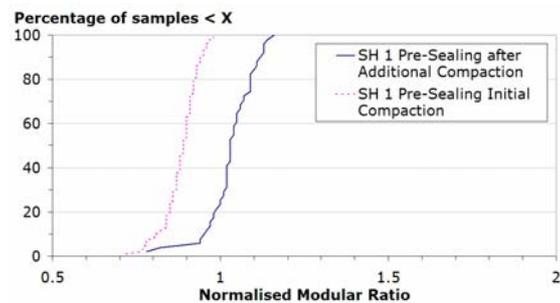
Figure 5. Increase in Normalised Modular Ratio with Additional Compaction.
