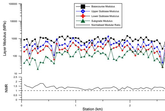
Figure 3. Moduli and Normalised Modular Ratios for Variable Subgrade.
