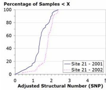
Figure 10. LTPP Site 21. Cumulative Distribution of HDM Modified Structural Number (SNP) in Successive years.
