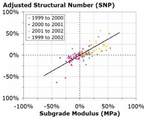
Figure 12. Trend showing change in Adjusted Structural Number (SNP) versus change in Subgrade Modulus ( $E_s$ ) for all LTPP sites.
