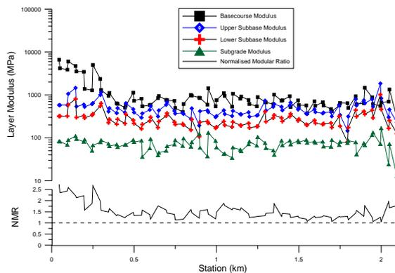
Figure 2. Back-calculated Moduli and Normalised Modular Ratios (NMR) for Firm Subgrade.
