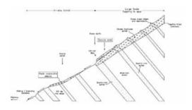
Figure 2. Cross-section of the rock avalanche area.
