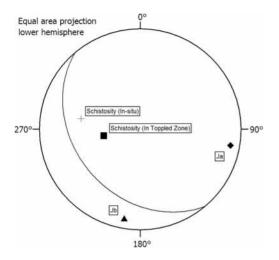
Figure 4. Lower hemisphere, polar, equal area stereoplots of mean attitudes of rock defects. The great circle indicates average dip of slope surface in the rock avalanche source area.
