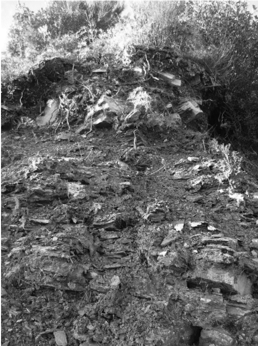
Figure 5. Highly fragmented but relatively un-disaggregated schist with fine gravel to boulder sized clasts, exposed above State Highway 6.
